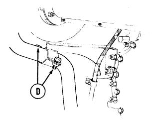
4. On later model transmissions, use 3/4 inch socket and extension to remove two nuts (D) securing bracket to transmission.
