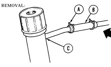
1. Using hose clamp pliers, loosen clamp (A).
