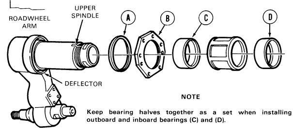
14. Coat inner and outer races of outboard bearings (C) with grease. Install inner race on spindle. Install outer race over it.
