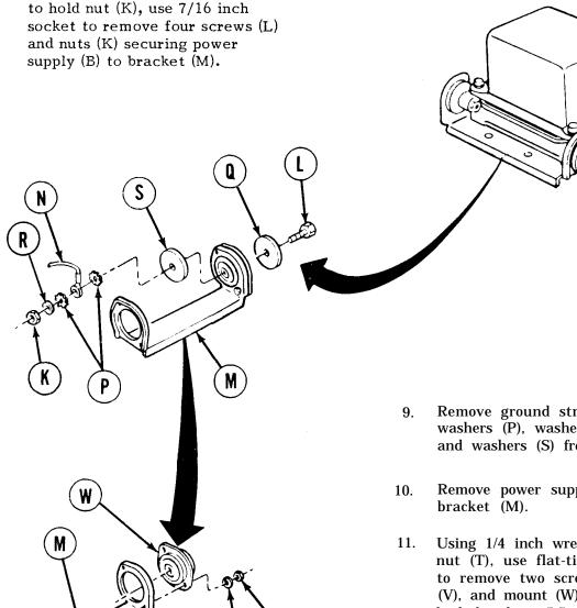
Remove ground strap (N), two lockwashers (P), washer (Q), washers (R), and washers (S) from bracket (M).
