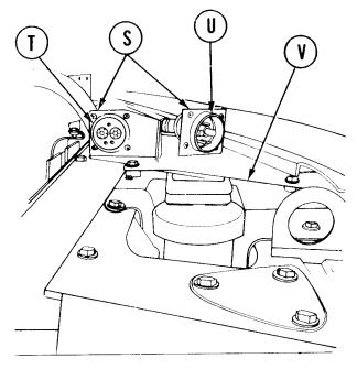
6. Using screwdriver and 3/8 inch wrench, remove eight screws, lockwashers, and nuts (S). Remove electrical connectors (T) and (U) from connector bracket (V).
