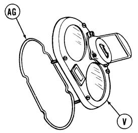
14. Apply adhesive to headlight cover seal (AG) and insert on headlight cover (V).
