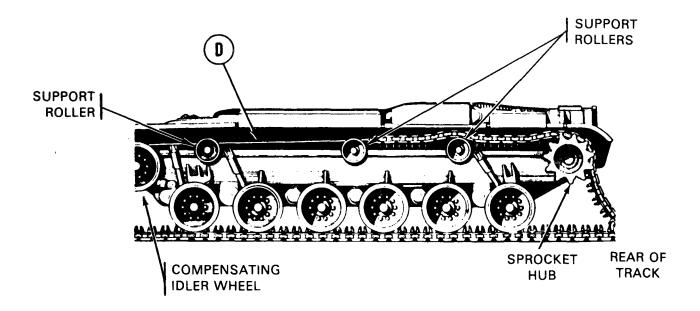
22. With rope still attached to rear of track, pull rope forward over all three support rollers and compensating idler wheels.
