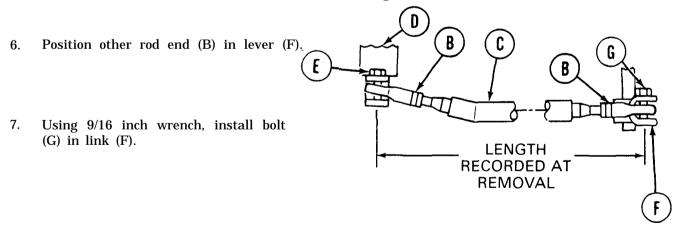
8. Test operation of steering control rod (C) linkage (TM 5-5420-202-10).
