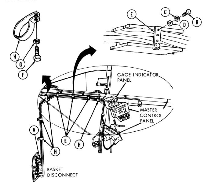
4. Install and connect harness assembly (A) at basket disconnect (page 10-296.71).
