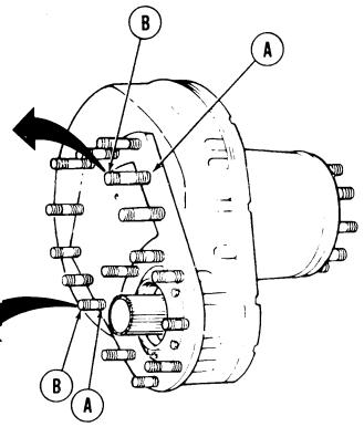
2. Apply penetrating oil to base of stud (A). Sharply tap head of stud (B) with hammer. Using pipe wrench (F), remove broken stud (B).
