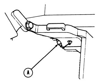
1. Disconnect connector (A) of left air cleaner blower lead.
