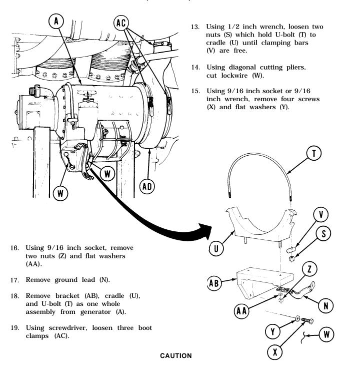
Boot (AD) is easily damaged. Be careful to prevent ripping or puncturing boot (AD).
