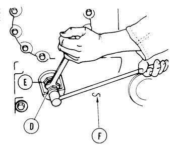
3. Using torque wrenchand 1-1/16 inch socket on adjusting screw (D), torque adjusting screw (D) 25-30 lb-ft  $(34-41 \text{ N}\cdot\text{m})$ .
