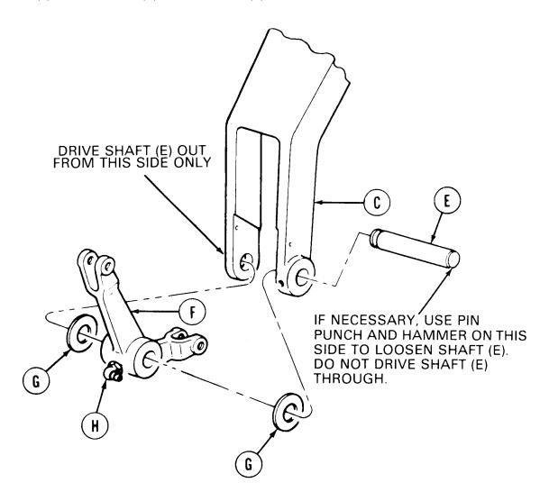
6. Using 3/8 inch open end wrench, remove grease fitting (H) from link (F).
