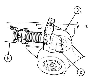
Remove adjusting link (F) from bearing (C) in number 1 roadwheel support arm (D).
