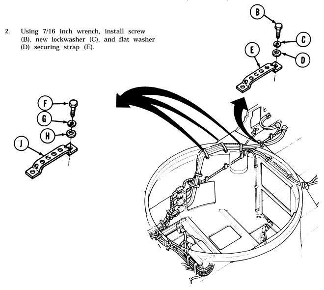
3. Using 7/16 inch wrench, install two screws (F), new lockwashers (G), and flat washers (H) securing three straps (J).
