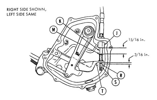
ONE-PIECE LEVER AND PAWL WITH TWO JAM NUTS
