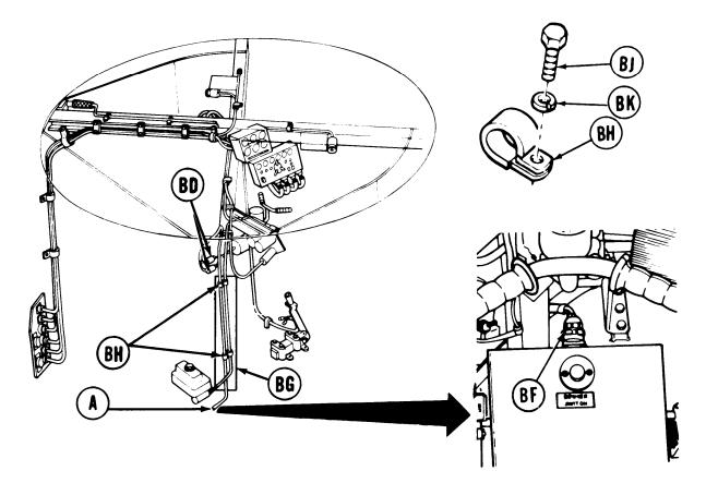
32. Using 7/16 inch socket, secure wining harness assembly (A) to vertical post (BG) located to left and forward of driver's seat, with clamps (BH), screws (BJ), and new lockwashers (BK).
