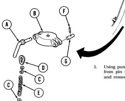
5. Using punch and hammer, remove pin (F) from pin (G) securing cover (B) to vehicle and remove pin (G) and cover (B).
