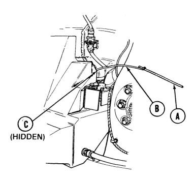
2. Attach wire (B) extending from tube (C) at the engine compartment tightly to the forward end of new control assembly (A).
