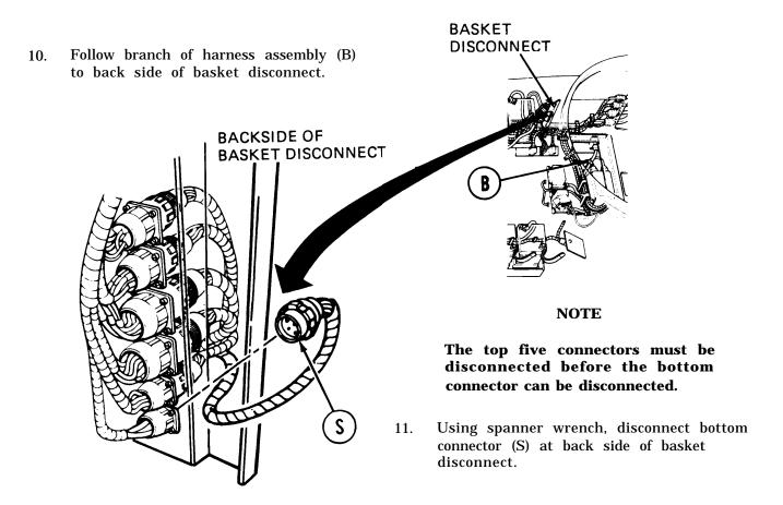
12. Remove wiring harness assembly (B) from vehicle.
