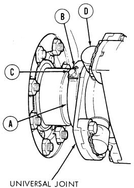
4. Remove ring (quick-disconnect) assembly (A) from universal joint (D).
