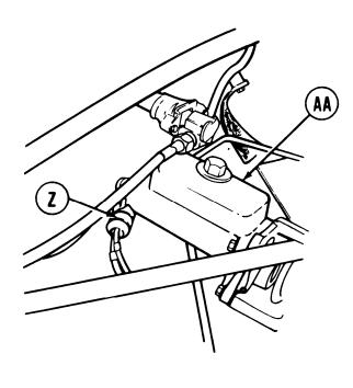
8. Connect connector (Z) (CKT 75,75) to brake master cylinder (AA).
