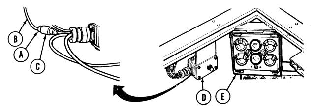
2. Route replacement hull intermediate lead assembly (B) beneath cable retaining straps from dust detector warning light box (D) to behind instrument panel cluster assembly (E) and along smoke lead (F) under floor up to starter cable connector (G).
