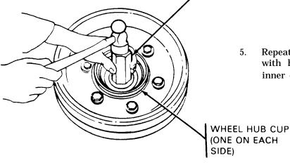
5. Repeat steps 1 through 4 using hammer with handle and remover-replacer to seat inner cup (C) in hub (B).
