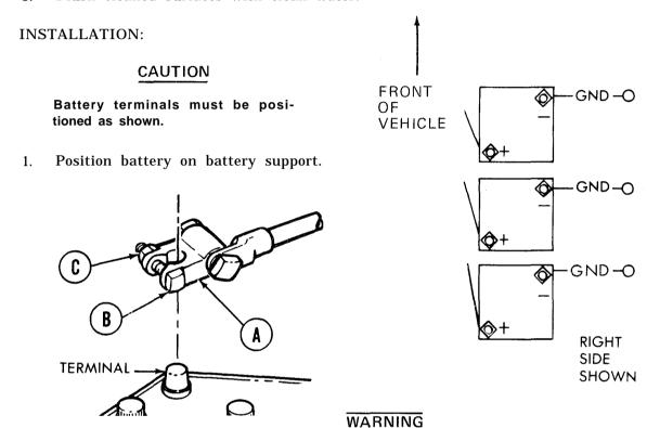
Do not let wrench handle touch hull metal while installing negative battery adapter (A). Arcing could occur and personnel could be burned.
