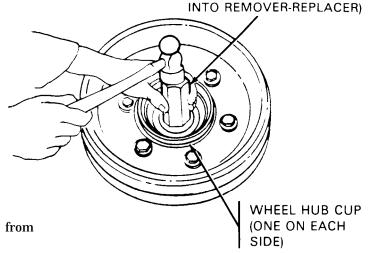
Using hammer, tap handle to drive outer
