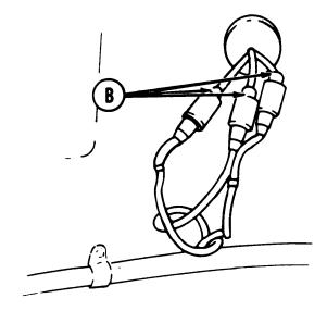
3. Disconnect two connector leads (C) from right blackout taillight/stoplight.
