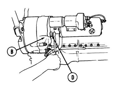
4. Using special wrench, secure last nut (D) onto stud.
