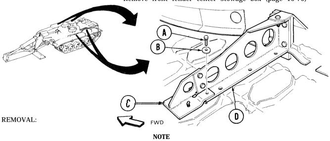
Left No. 3 fender support is shown, right No. 3 fender support replacement is similar.
