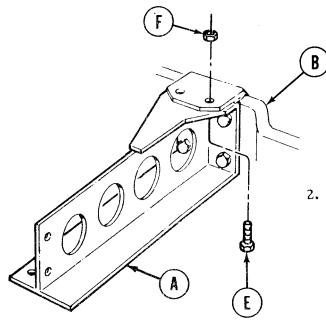
Using 3/4 inch socket and 7/8 inch wrench, secure top flange of support (A) to top of hull support with two screws (E) and nuts (F).
