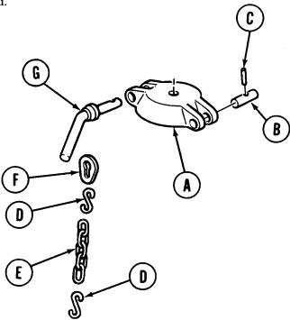
6. Move handle (G) in and out of cover (A) two or three times to make sure handle (G) does not stick in cover (A).
