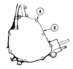
3. Move brake control bellcrank, at top center of transmission, to release position as shown.
