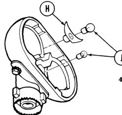
**4.** Using fingers, install reflector (H), and install two bulbs (J) by pushing in and twisting them clockwlse. Large bulb with reflector (H) goes on top.
