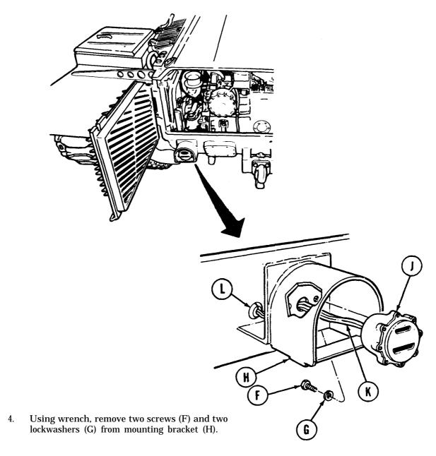
5. Remove taillight (J), pulling three taillight leads (K) through rubber grommet (L).
