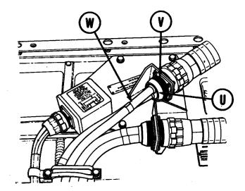
8. Using slip joint pliers, unscrew retaining nut (U) from shell (V). Slide retaining nut (U) back along cable assembly (W).
