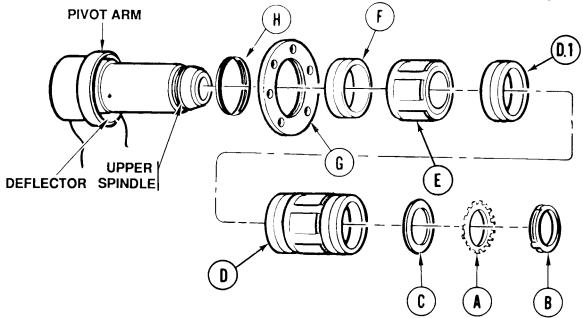
5. Slide oil seal retainer (G) off upper spindle.
