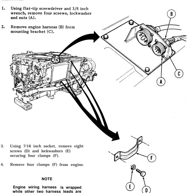
Separate and remove engine wiring harness (B) from top of engine.
