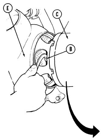
7. Using special box wrench, tighten six nuts (B).
