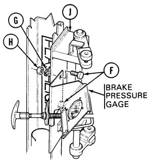
7. Install one bolt (F), washer (G), and nut (H) finger tight to support gage bracket.
