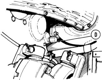
. Using 1 inch wrench, remove brake adjusting worm cap (D).
