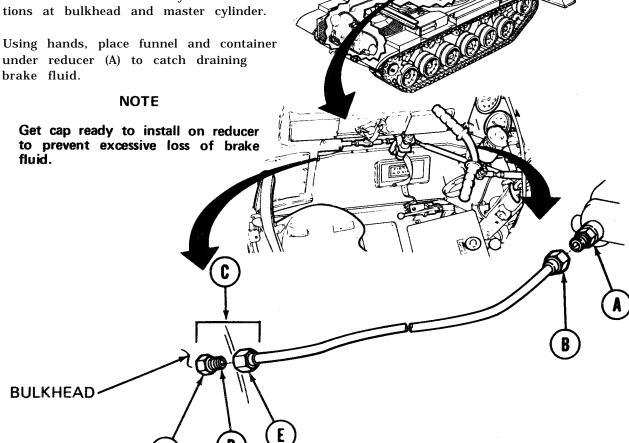
Using 13/16 inch wrench to hold reducer 3. (A), use 11/16 inch wrench to remove tube connecting nut (B). Cap reducer (A).
