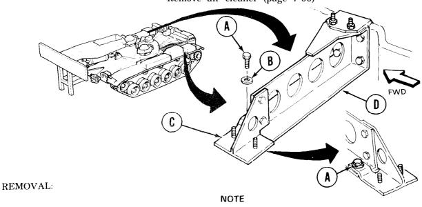
Left No. 4 fender support is shown; right No. 4 fender support replacement is similar.
