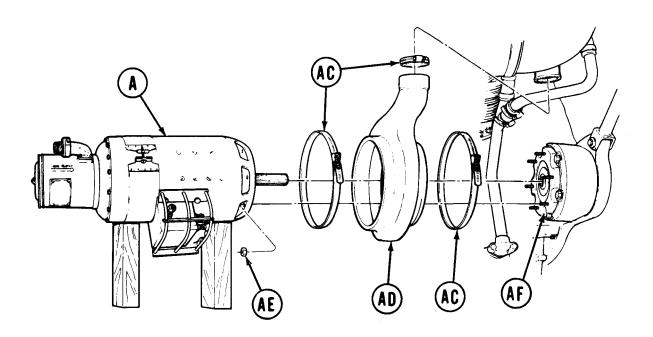
22. Using two technicians, rotate generator (A) counterclockwise until openings in flange are alined with nuts (AE).
