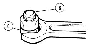
1. Apply penetrating oil to base of stud (A). Thread two hex nuts on stud (B) and jam the nuts. Sharply tap head of stud (B) several times with hammer. Turn lower nut (C) to remove stud (B).
