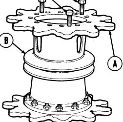
4. Use three 5/8-18 UNF bolts. Screw them into three threaded holes in sprocket (A).
