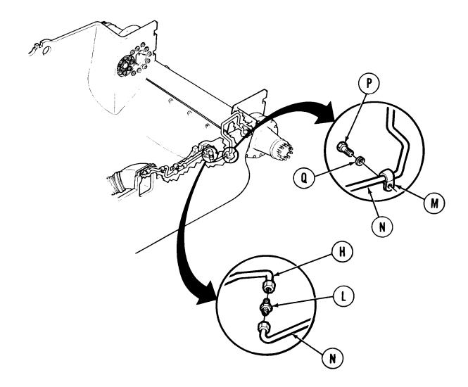
15. Using 7/16 inch wrench, install and tighten screws (P) and new lockwashers (Q) securing clamps (M) to hull.
