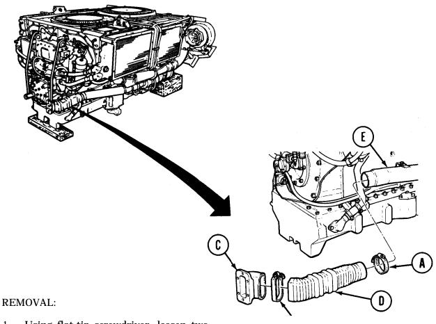
1. Using flat-tip screwdriver, loosen two clamps (A) and (B).
