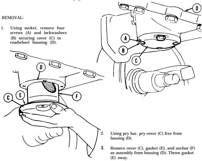
TORSION BAR ANCHOR REPLACEMENT (Sheet 2 of 3)
