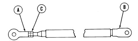
2. Using torque wrench and crowfoot adapter, tighten nut (C) against rod end bearing (A) to 16-18 lb-ft (23-24 N·m).
