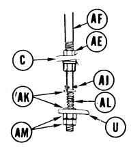
32. Position lever assembly (U) on control assembly (AF) and thread two nuts (AM) on control assembly finger tight.
