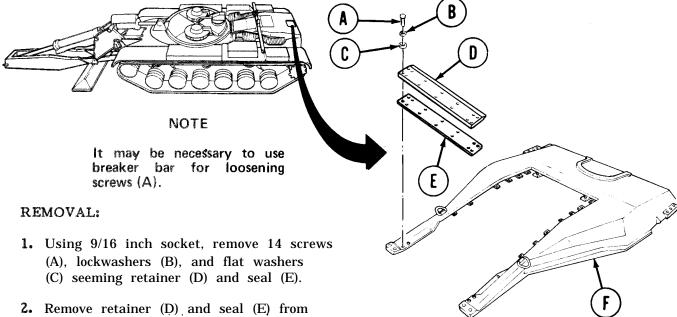
2. Remove retainer (D) and seal (E) from top deck (F).
