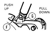
4. Aline lower shock absorber yoke (F), with roadwheel support arm (G). Aline keyways by pushing up or pulling down on yoke.
