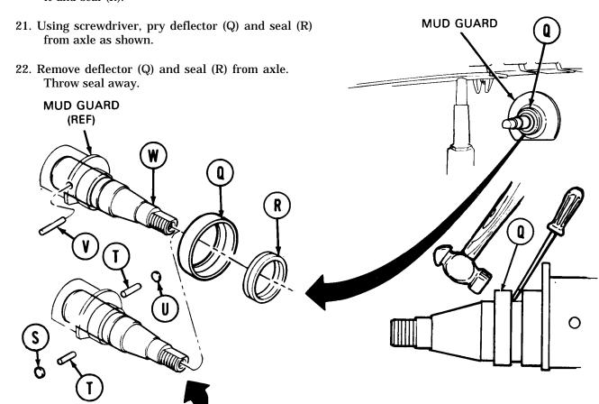
23. On left front support roller ONLY, using 3/16 inch alining punch and hammer, tap around edges of plug (S) until plug can be pried free with screwdriver.
