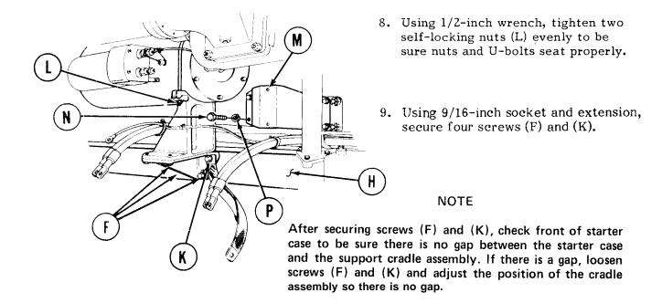
10. Position low voltage relay solenoid bracket (M) on engine oil pan (H) and using 1/2-inch socket and extension, secure low voltage relay solenoid bracket (M) to engine oil pan (H) with four screws (N) and lockwashers (P).
