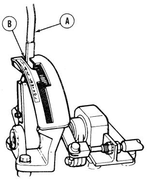
5. At driver's station, move transmission shift lever (A) to P position (B).
