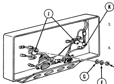
Using socket, install two lockwashers (F), flatwashers (G), and nuts (H) securing two harness junctions (J) to panel.
