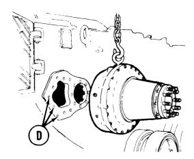
Using socket or offset link, install 17 new self-locking nuts (E).
