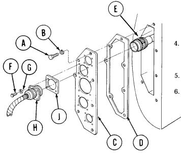
4. Using screwdriver, remove 16 screws (F) and lockwashers (G) securing four receptacles (H) and gaskets (J) to mounting plate (C).
