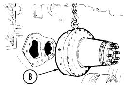
Keeping hoist chain tight, slowly pull final drive (B) from hull.
