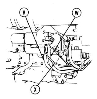
6. Using 3/4 inch wrench, secure male connector cables (V) and (W) and light cable (X) with lockwasher and nut.
