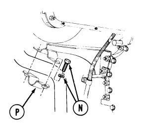
15. On later models, use 3/4 inch socket to tighten two nuts (N).
