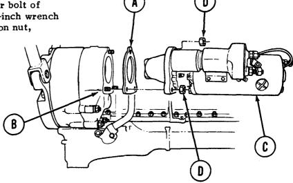
3. Install lower nut (D) and bolt in same way as upper nut and bolt in step 2.
