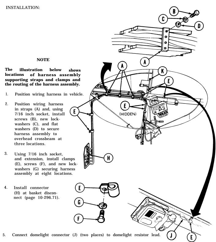
6. Connect gas particulate connector (K) to gas particulate lead.
