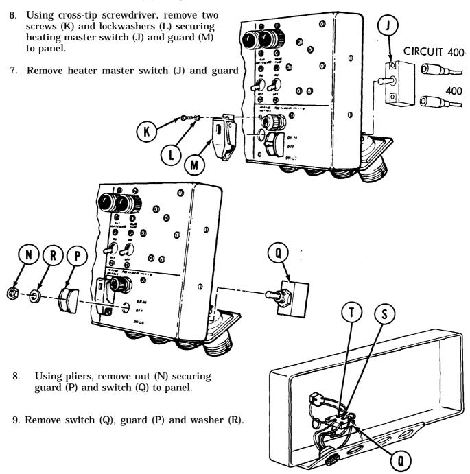
10. Using flat-tip screwdriver, remove five screws (S) and lockwashers (T) securing six electrical leads and jumper wire to switch (Q).
